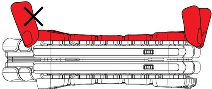
2. Gently remove both keyboard halves by grasping the keyboard by the metal body and lifting them out of the case. Do not grasp the keyboard by its keys when handling.
